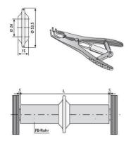
Swellable SD type water stop to prevent the ingress of water. Fitted using BETOMAX® SD installation pliers.
