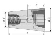
Metal-plastic cone for multiple use in concrete. Compatible with Uni-rods.
