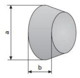
For closing conical holes. Bonded in with two-component adhesive. 1 kg of adhesive is sufficient for approx. 40 B15 plugs.
