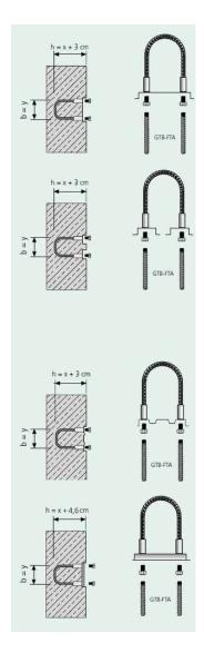
The combined version COMAX® GTB is a factory-prefabricated screw connection element for the transmission of static and dynamic loads.
