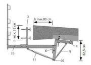
For wide cantilevered cap cornices in bridge construction.
