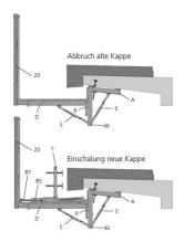
New renovation bracket with renovation ledger.
