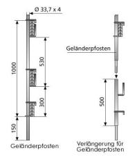
Complies with the safety rules for lateral protection and roof safety barriers as a means of safeguarding against falling (GB-I 807 of October 2002). According to DIN EN 12811.
