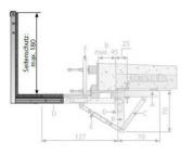
Accessory for the GK-2000 system, alternative to the BX guardrail as fully planked safety rail from structures above and under rail and road structures, e.g. electric railwaytracks and motorways.
