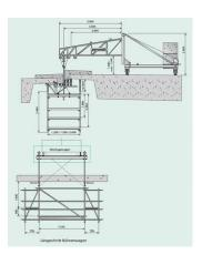
This combination is used especially in the area of the central cornice. The stage platform offers ideal conditions for assembly work and visual inspections under the bridge. The flow of traffic on the side of the bridge that is being used is not affected.
