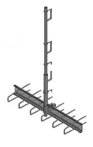
Railing post holder for holding the BETOMAX® railing post on the edges of ceilings and bridge superstructures made of concrete in conjunction with the plug socket that was concreted in beforehand.
