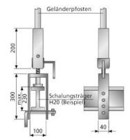
Clampable railing post holder. Suitable for wooden beams and steel profiles.
