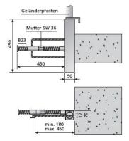
Guardrail post holder for accommodating BETOMAX® guardrail posts on the superstructure edges of bridges.
