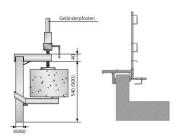
Clampable railing post holder for vertical and horizontal component edges.
