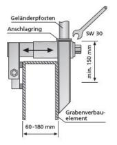
Clampable railing post holder for use on trench shoring elements. Suitable for element and wall thicknesses between 60 and 180 mm.
