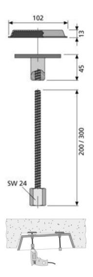
With the KNACKER®, even complicated or particularly firmly adhering bowl elements can be easily loosened. The hardened lid allows the KNACKER® to be used several times.
